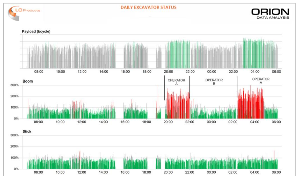
Figure 1 - Daily status report showing sudden and considerable changes in fatigue duty rate
